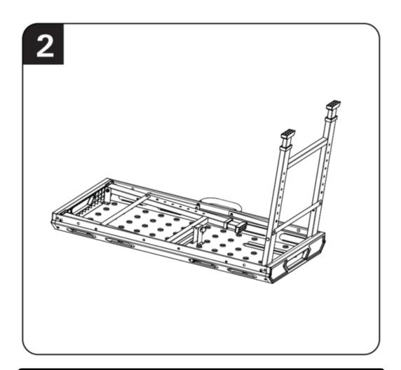
• Raise one table leg. Make sure the supporting braces are attached firmly to the table leg so that the will not collapse. Make sure the fasteners are fully engaged and secured to the legs and the table.
