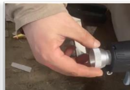
Install Cleaning Nozzle
