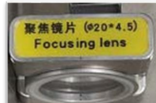
Focus Lens Assembly
