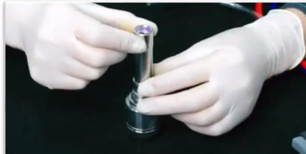
Collimating Lens Assembly Removed from Gun
