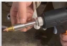
Remove Focus Tube
