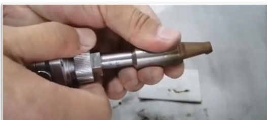
Focus Tube Adjustment
