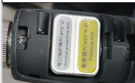
Protective and Focus Lens
