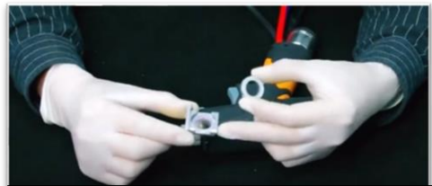
Protective Lens Replacement
