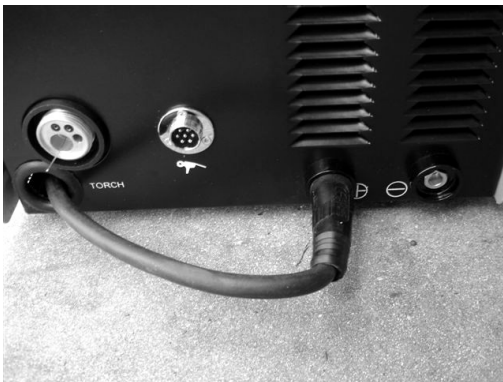
Image 2c. Machine set for MIG operation
