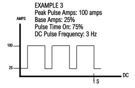
Setting up the pulse is not a process where a fixed adjustment procedure can be assigned or rigidly recommended. Changes to frequency, balance, and time will skew the final result. A slow pulse with a equal 50% pulse time on and somewhere around a 50-75% Pulse Base Amp setting is typically used to help with timing the addition of filler metal to the weld puddle. A higher pulse frequency level that is combined with variations in Pulse Time On and a narrow/wider ratio can be used to prevent burn
