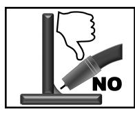
**Characteristics:** Concave weld, poor filling, possible undercutting resulting in weak weld.
