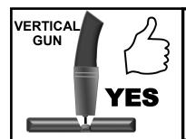
Correct Technique: The gun is held in a near vertical position. A variance of 5 degrees or less is acceptable from side to side. The purpose is to prevent the arc from being concentrated on one side of the weld joint or the other. This balances the heat on both sides of the joint and keeps the bead centered. Don't confuse this with push or pull angle in the travel direction.
