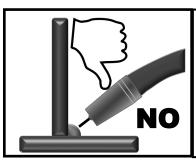
Characteristics: Small Convex weld possibly with bulging sides/cold lap and/or an inconsistent arc. Possible Causes: Not enough Voltage or Amperage. If weld is ropy and thin without bulging at the toes, travel speed is too fast or using a pull technique. Remedy: Increase voltage and amperage, slow down to fill joint more. Use push technique.
