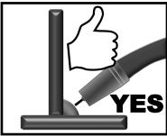
Proper Weld Characteristics: Weld is slightly convex, weld legs (vertical and horizontal width of weld) are equal in length and match the thickness of the metal being welded. No traces of undercutting, Proper tie in of the weld at the toes with no cold lap. Weld is not overfilled or under-filled with no significant amounts of spatter, soot or contaminates around weld. Weld is not oxidized and is bright.
