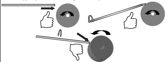
Do not grind the Tungsten parallel to wheel face or an unstable arc will result.
