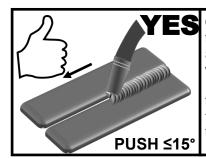
Correct Technique: The gun can be angled toward the front of the weld when traveling forward. This angle should not exceed 15 degrees. This provides a wider and generally more pleasing weld. However it is shallower penetrating. This method typically allows a much better view of the arc. Use for most types of welding unless deeper penetration must be achieved.
