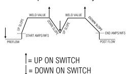
4T Torch Operation Effect on Weld Cycle.
