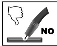
**Problem:** Gun is not being held vertical from side to side. Wire is not being directed to the center of the puddle. This concentrates heat on one side of the joint and results in poor fusion on the neglected side. It also can create more buildup on one side of the joint than the other.
