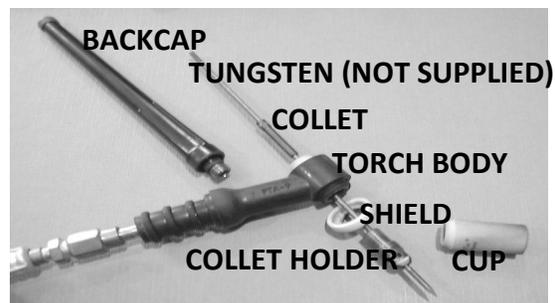
pictured below (handle is removed for further detail): To use the TIG lift arc, flip the switch toward the TIG icon on the welder. Adjust welding current with the Amp control knob to desired amp level. Make sure the tank is open and the regulator is adjusted for 10-
