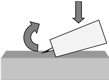
3. After contact with the metal, quickly rock the torch back so that the tungsten breaks contact with the metal.
