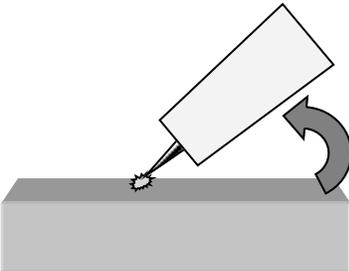
4. An arc should form. As the arc grows raise the cup up off the metal and slowly rotate the torch into welding position.
