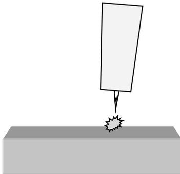
3. An arc should form, after a slight spark or snap sound. If arc does not start, repeat it and move tungsten closer to metal.
