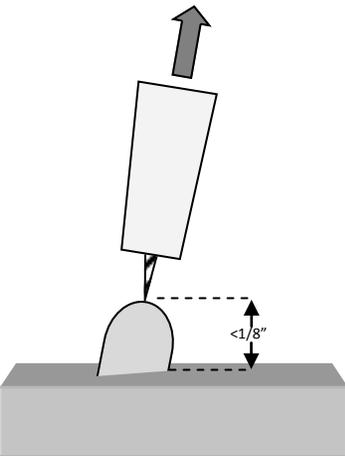
5. Leave 1/8" or less gap between the tungsten tip and the metal.
