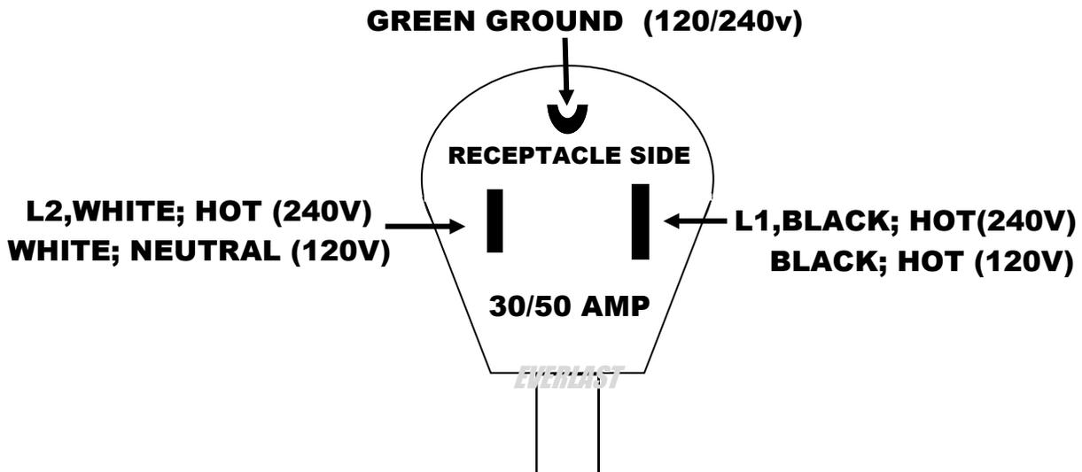
**IMPORTANT: WHILE USING THE POWERARC 140 ST/160 STH WITH A 120V POWER SUPPLY, BE SURE TO USE THE WHITE WIRE AS THE COMMON/NEUTRAL, THE BLACK AS THE HOT, AND THE GREEN AS THE GROUND OR MALFUNCTION/DAMAGE MAY OCCUR.**
