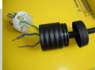
Above left is a 4 prong male plug (250VAC/30AMP), plug cap, rubber cap seal and the cord from the welder. Use this same procedure on 3 prong (250VAC) plugs (there's no neutral on the 250VAC "three" prong plugs). The above right picture shows the seal and cap on the cord and the ground wire connected to the ground terminal, note the green on the ground terminal (green wire goes there).
