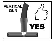
**Correct Technique:** The gun is held in a near vertical position. A variance of 5 degrees or less is acceptable from side to side. The purpose is to prevent the arc from being concentrated on one side of the weld joint or the other. This balances the heat on both sides of the joint and keeps the bead centered. Don't confuse this with push or pull angle in the travel direction.
