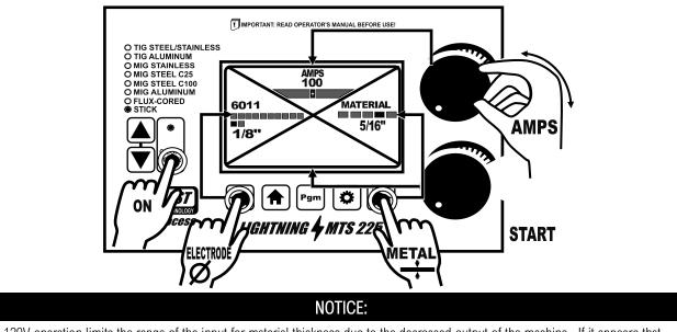
120V operation limits the range of the input for material thickness due to the decreased output of the machine. If it appears that some X menu input selections for material thickness are limited, double check to see if the unit is plugged into 120V. Stick Performance may be affected in 120V mode. Less arc force is available to maintain a steady arc.
