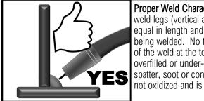
**Proper Weld Characteristics:** Weld is slightly convex, weld legs (vertical and horizontal width of weld) are equal in length and match the thickness of the metal being welded. No traces of undercutting, Proper tie in of the weld at the toes with no cold lap. Weld is not overfilled or under-filled with no significant amounts of spatter, soot or contaminates around weld. Weld is not oxidized and is bright.
