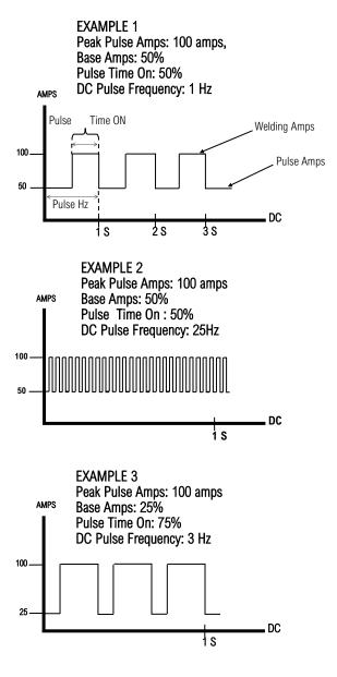
Setting up the pulse is not a process where a fixed adjustment procedure can be assigned or rigidly recommended. Changes to frequency, balance, and time will skew the final result. A slow pulse with a equal 50% pulse time on and somewhere around a 50-75% Pulse Base Amp setting is typically used to help with timing the addition of filler metal to the weld puddle. A higher pulse frequency level that is combined with variations in Pulse Time On and a narrow/wider ratio can be used to prevent burn
