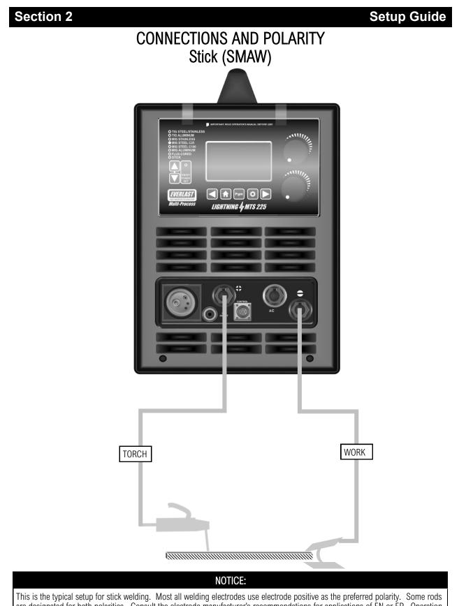
This is the typical setup for stick welding. Most all welding electrodes use electrode positive as the preferred polarity. Some rods are designated for both polarities. Consult the electrode manufacturer's recommendations for applications of EN or EP. Operation with old or improperly kept welding electrodes will affect performance. If difficulty is encountered welding with a particular class of rod, try changing to another brand.
