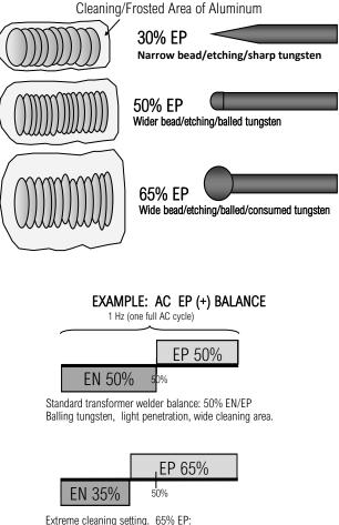
Shallow penetration, balling tungsten, excessive cleaning area.
