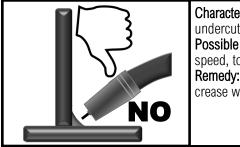
Characteristics: Concave weld, poor filling, possible undercutting resulting in weak weld. Possible Causes: Voltage too high, not enough wire speed, too short of wire stick out, wrong gun angle. Remedy: Decrease voltage, use push motion, increase wire speed.
