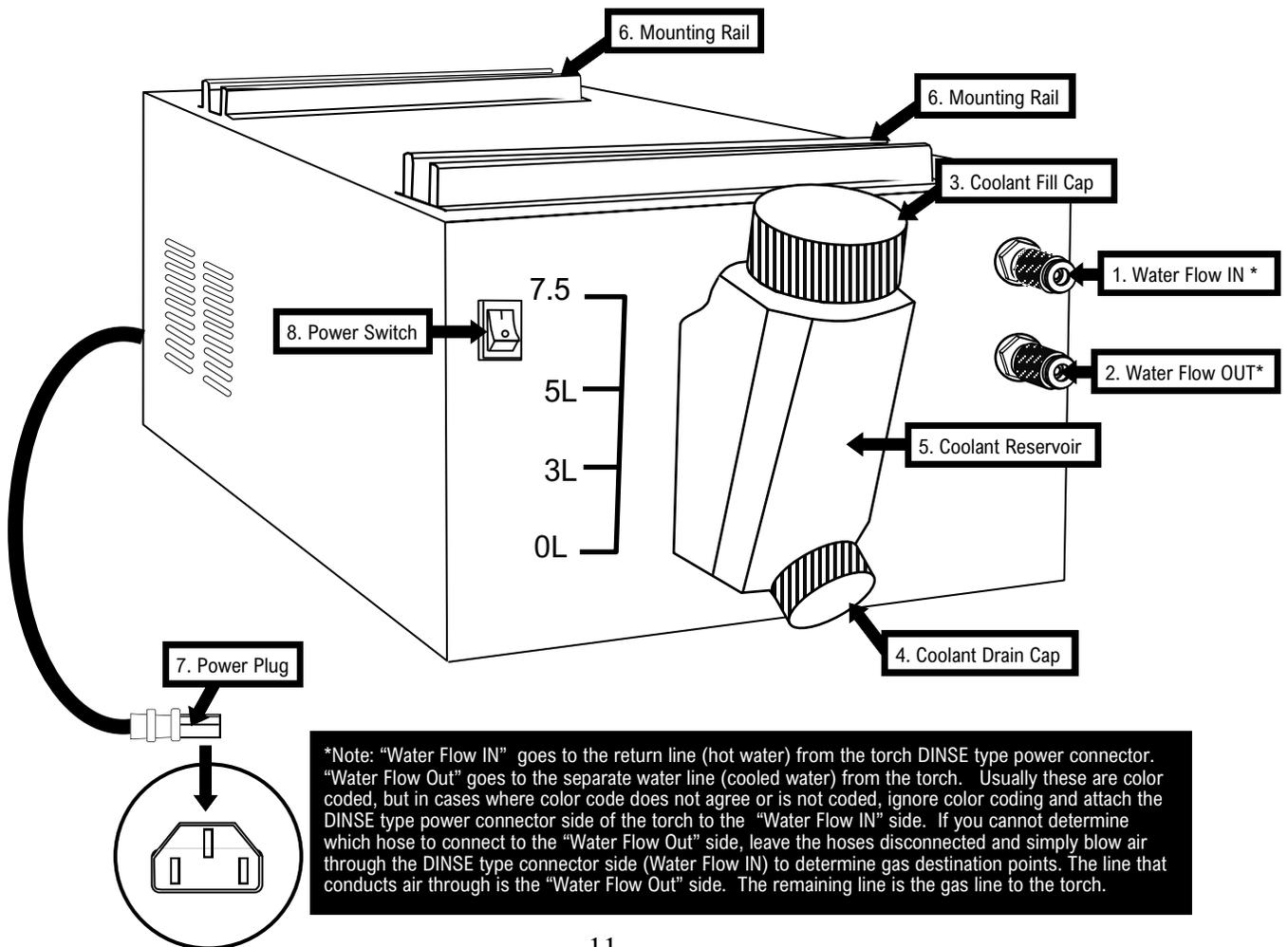
**2.1 Basic Features.** The Everlast PowerCool 400 is rated for 400 amps of cooling for either TIG or MIG welders. It is designed to be stacked with the PowerTIG 315LX, PowerTIG 350EXT, and the PowerMTS 252STi, and Lightning 275. It will work with all machines in the Everlast lineup equipped with a rear Power Plug, but modifications will be required to the top rails and will require the end user to refit and make the necessary adjustments.
