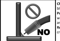
**Characteristics:** Concave weld, poor filling, possible undercutting resulting in weak weld. **Possible Causes:** Voltage too high, not enough wire speed, too short of wire stick out, wrong gun angle.
