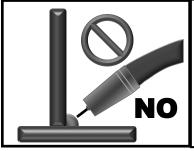
**Characteristics:** Small Convex weld possibly **with** bulging sides/cold lap and/or an inconsistent arc. **Possible Causes:** Not enough Voltage or Amperage. If weld is ropy and thin without bulging at the toes, travel speed is too fast or using a pull technique.
