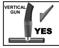
**Correct Technique:** The gun is held in a near vertical position. A variance of 5 degrees or less is acceptable from side to side. The purpose is to prevent the arc from being concentrated on one side of the weld joint or the other. This balances the heat on both sides of the joint and keeps the bead centered. Don't confuse this with push or pull angle in the travel direction.
