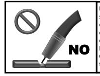
**Problem:** Gun is not being held vertical from side to side. Wire is not being directed to the center of the puddle. This concentrates heat on one side of the joint and results in poor fusion on the neglected side. It also can create more buildup on one side of the joint than the other. **Correction:** Hold the gun so that the angle of the neck stands perpendicular from side to side.
