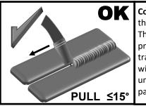
**Correct Technique:** The gun is angled toward the back of the weld when traveling forward. This angle should not exceed 15 degrees. This provides a narrower but more deeply penetrating weld. Use this method when Flux Core wire is being used. Use this method where the unit may be reaching its maximum welding capacity. Not for use with Aluminum wire.
