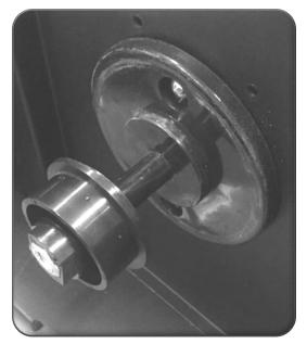
Above Image: Correct assembly of wire carrier for use with 4" spools.
