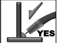
**Proper Weld Characteristics:** Weld is slightly convex, weld legs (vertical and horizontal width of weld) are equal in length and match the thickness of the metal being welded. No traces of undercutting, Proper tie in of the weld at the toes with no cold lap. Weld is not overfilled or under-filled with no significant amounts of spatter, soot or contaminates around weld. Weld is not oxidized and is bright.
