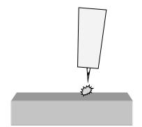
3. An arc should form, after a slight spark or snap sound. If arc does not start, repeat it and move tungsten closer to metal.
