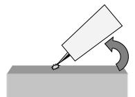
4. An arc should form. As the arc grows raise the cup up off the metal and slowly rotate the torch into welding position.
