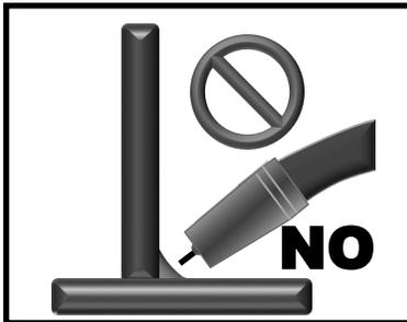
**Characteristics:** Concave weld, poor filling, possible undercutting resulting in weak weld.
