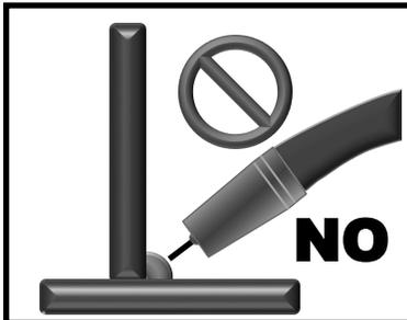
**Characteristics:** Small Convex weld possibly with bulging sides/cold lap and/or an inconsistent arc.
