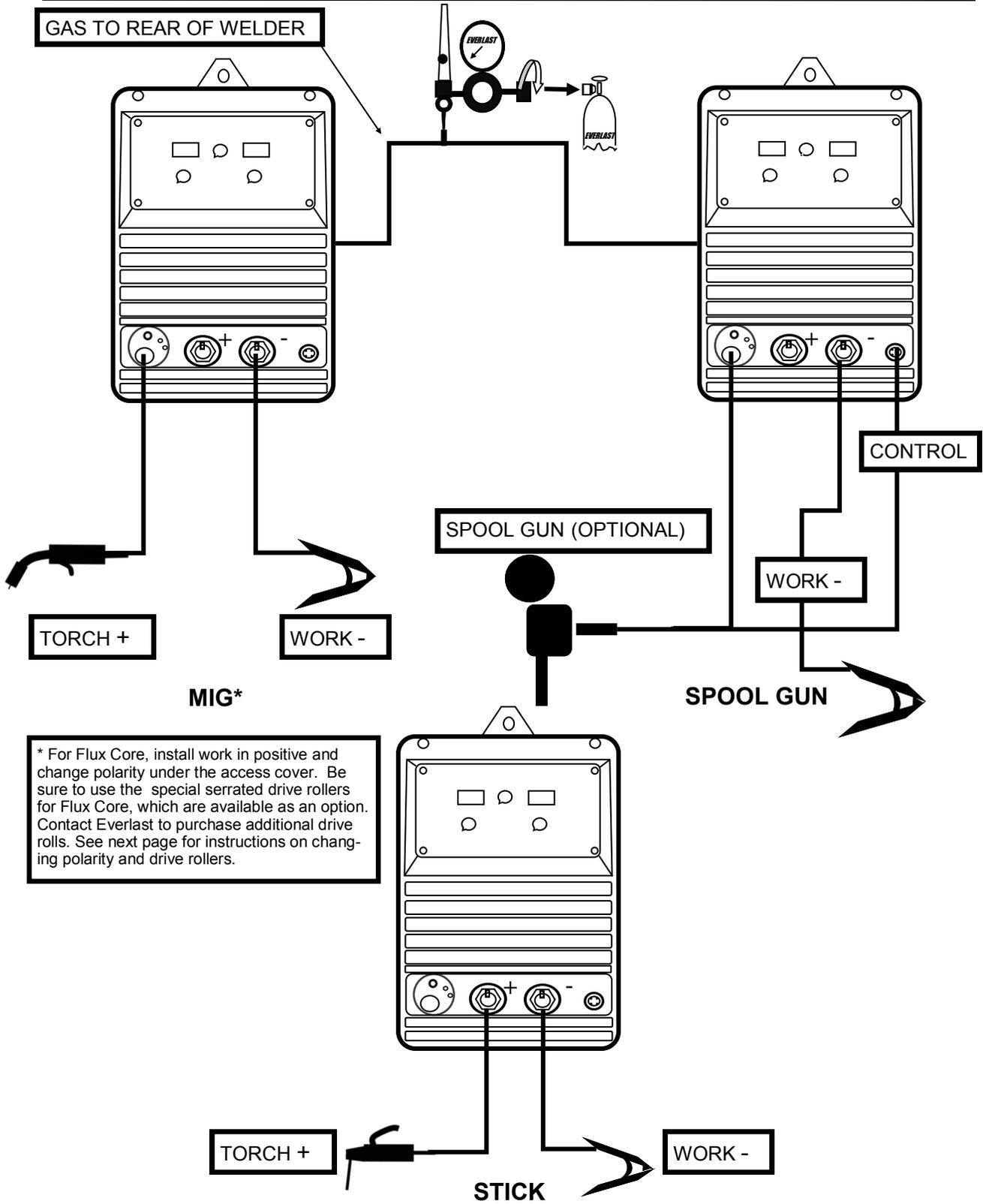
\* For Flux Core, install work in positive and change polarity under the access cover. Be sure to use the special serrated drive rollers for Flux Core, which are available as an option. Contact Everlast to purchase additional drive rolls. See next page for instructions on changing polarity and drive rollers.
