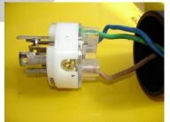
Above left, is ground connected and one hot leg (X). Above right is the other hot leg connected (Y). There is no neutral wire on the 220VAC welder, so the (W) neutral terminal is not used. At this point screw on the cap, push on the rubber seal and back to reading the manual. This connector was picked as it will hook to most generators and twist locks in the socket so the cord will not fall out.
